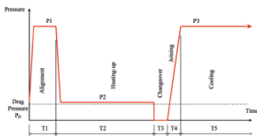
Graphic 2: Process stages of butt welding
